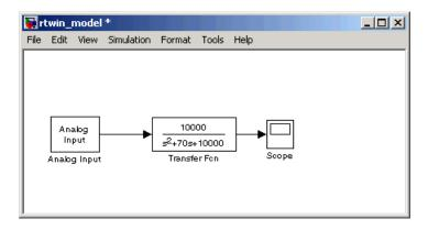
You next task is to enter parameters for the Analog Input block. See "Analog Input Block" on page 4-10.
